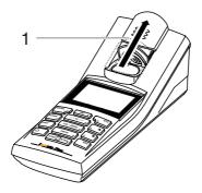
Inserting a 28 mm cell
