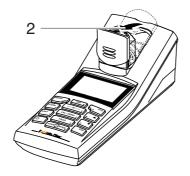
2 Pull upwards the height adapter (3). The cell shaft is extended.
